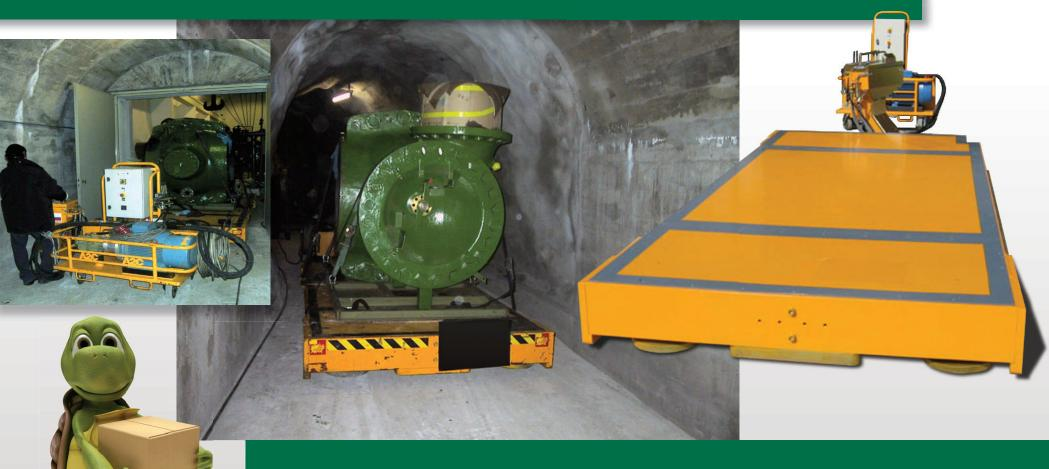
The TURTLE moves and places heavy loads where a forklift, overhead hoist or mobile crane cannot reach.
