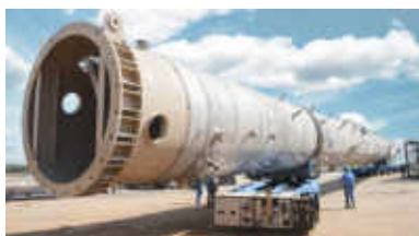
SCHEUERLE-KAMAG K25 H PowerBooster transporting a long load on bolsters
