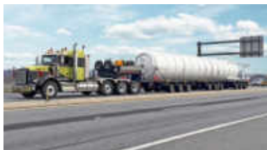
SCHEUERLE HighwayTrailer transporting a long load
