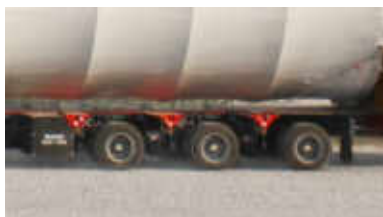
The proven hydraulically suspended pendulum axle technology ensures high tilting stability
