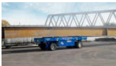
SPMT Light with steel girder for bridge construction
