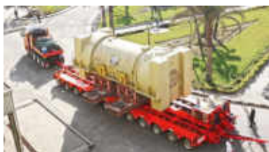
SCHEUERLE InterCombi transporting concentrated load
