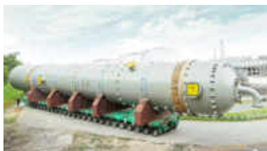
SCHEUERLE SPMT transporting splitter column
