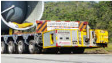
The PPU attached at the rear can vary its angle to adapt to road condition
