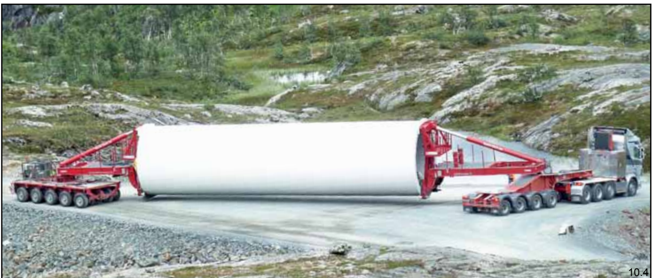
NICOLAS MDEL with the new wind tower adapter
