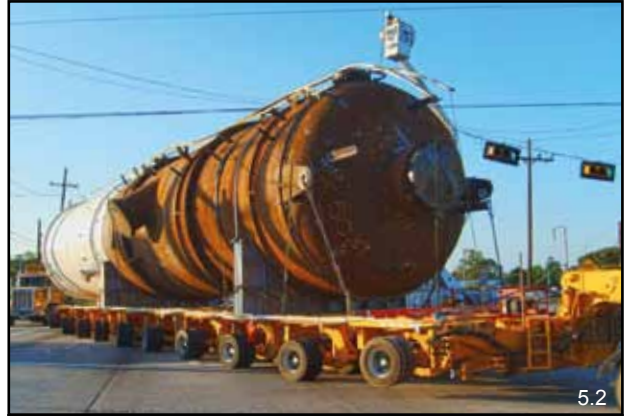
WideCombi as 10 axle semi-trailer
