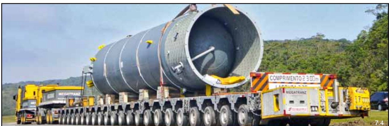
SCHEUERLE PowerBooster configuration
