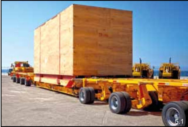
WideCombi with low bed deck
