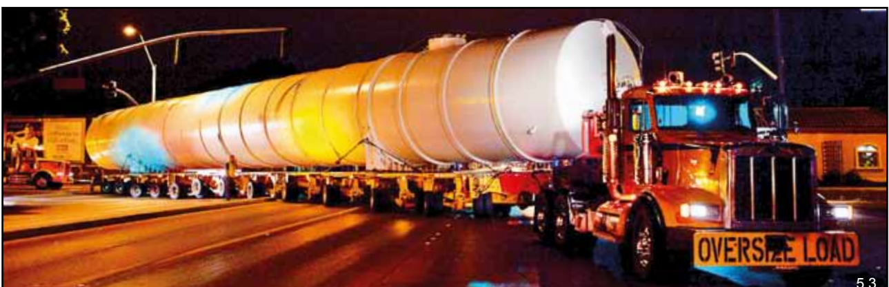
12 axle WideCombi W0 trailer combination
